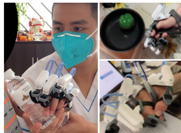
Training the weak upper limb to perform activities of daily living with a wearable hand robot.
